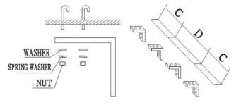
3.3.3 Set the mounting plate on the ceiling brackets and ensure safe & fixing (use the bolts attached to the ceiling brackets as Fig. Using the ceiling brackets to hang from the ceiling, the position of mounting plate can be adjusted in the limit of 100mm.
