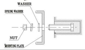
3.1.2 Fix the bolts in the proper position (Decide the position with the mounting plate and pour cement into the bolt holes.)
