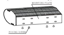
3.1.3 When the cement has freeze, fit the mounting plate (use the washer and nut according to the following)
