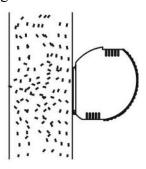
2.4 When the entrance is wider than the unit, it is recommended to install two or more units in parallel. In this case, provide 20-40mm gaps between the units.
