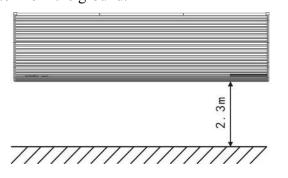
2.5 Don't allow gaps between the unit and the wall. When hanging it from the ceiling, using the enclosed ceiling braskets.
