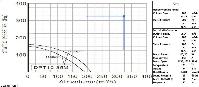
DPT fan design enables it's application in supply or exhaust ventilation systems for varios kind of ventilation needs.
