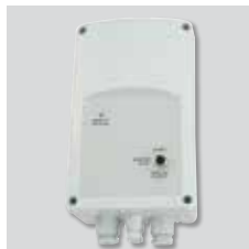
VAPZ Electronic single phase regulator that controls the fan speed with a simple contact (presence detector) or an analogical input, 0-10 V or 4-20 mA (from CO 2 probe or relative sensor).
