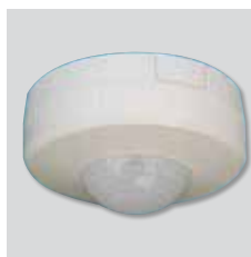
CPFL-S / CPFL-E Presence detector for ceiling mount, sensitive to infrared radiation by bodies in movement, with a 360° detecting angle. Power supply: 1-230 V.
